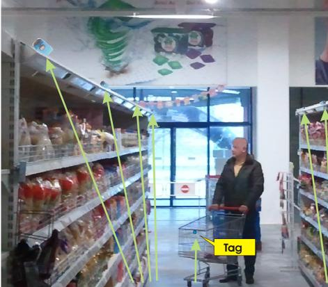
Hexamite Hx19 ultrasonic positioning tag is mounted on the cart. Hx19 positioning receivers are mounted on the top of the shelves
