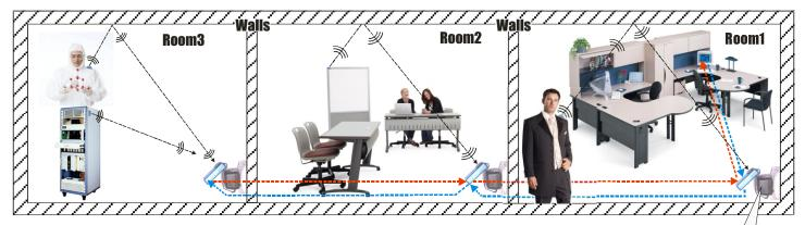
Above: the (license free) 2.4Mhz radio wave; travels along the red and blue lines through walls. and most non-metalic materials. Radio Frequency (RF) is used to relay messages room to room; towards the main server in room1, where tag time and location is stored and internet updated. The HabiTag ultrasound represented by the green lines, does not travel through walls. Hence; sonic-electromagnetism combination yields a highly reliable way, to located objects and people indoors.
